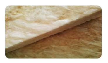
**Reduce Sound Transmission.** Exceptional soundabsorbing properties. Specially designed to reduce transmission of unwanted noise. This is ideal for drywall partition systems for rooms and offices in residential, commercial and industrial buildings.
