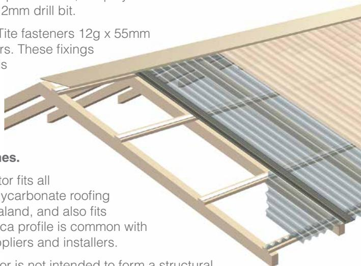
The Laserlite® Lap Connector fits all 76mm pitch corrugated polycarbonate roofing commonly used in New Zealand, and also fits Greca profile perfectly. Greca profile is common with New Zealand's Pergola suppliers and installers.
